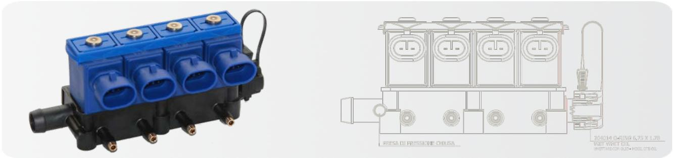
The injection unit ensures that the right quantity of gas is delivered into the intake manifold at the intake valves. The electronic injectors are opened in the right sequence and at the right time to suit the engine's ignition cycle.
